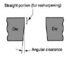
Fig.4: Angular ClearanceTypical values: 0.25° to 1.5° on each side**3.1** Design of Blanking tool:
