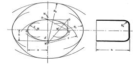
Fig.1:Blank Development for irregular shells.
