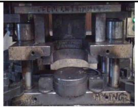
*Fig 9: Trimming Tool.* **3.19. Hole Flanging & 3.50 Flaring Tool design:**
